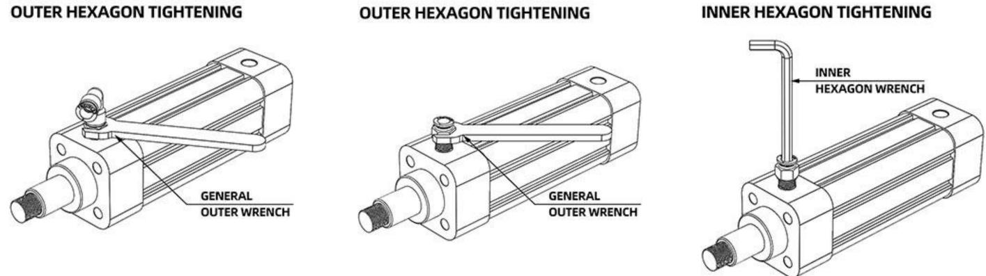
2.2.2 When loosen the fittings from equipment body, please use proper tool. After disconnecting, please clean the thread glue on equipment, otherwise the remaining thread glue will enter the equipment and cause damage.
